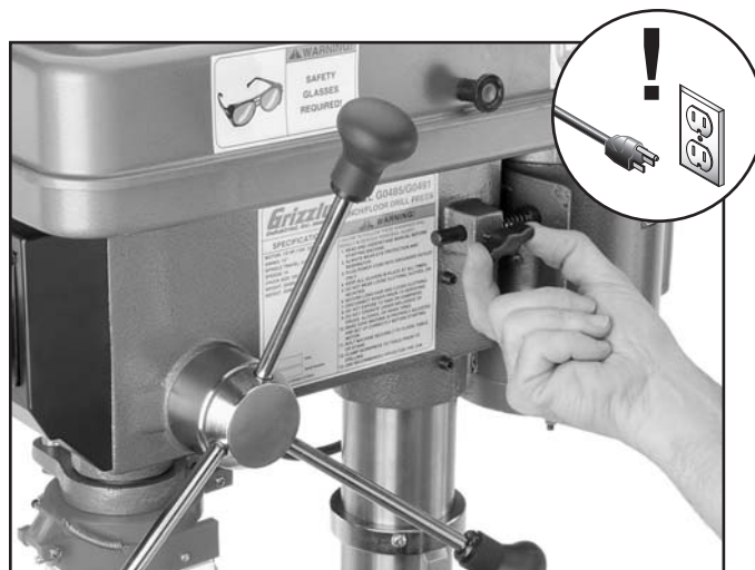
Figure 28. Loosening lock knob.
